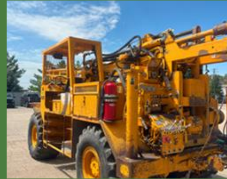
Conventional drill rig
