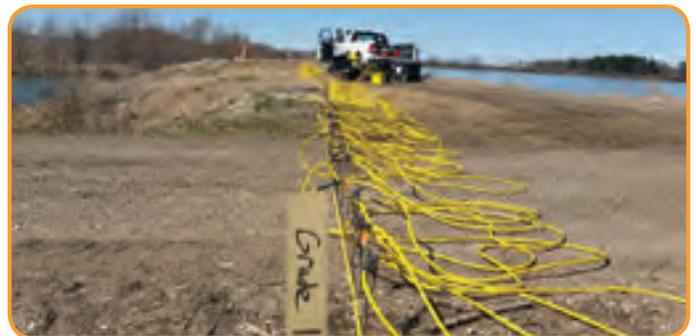
Shown here is a typical ERI survey layout consisting of 112 pins hammered into the ground connected by a cable.
