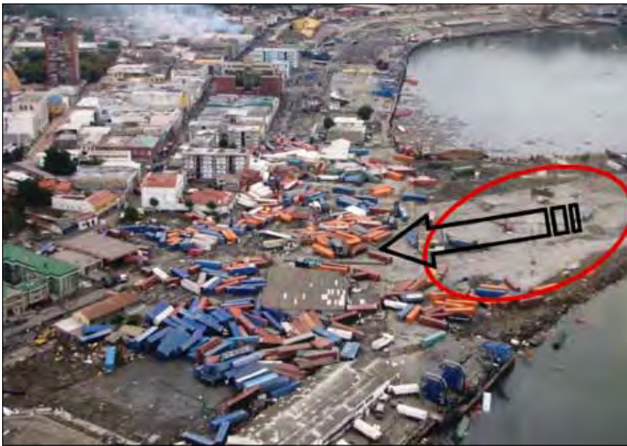
Figure 10. Talcahuano Harbor 3 days after the tsunami (photo: Intl. Federation of Red Cross Red Crescent Societies). Shipping containers were originally stacked in the area of the red ellipse and displaced up to 300 m in the direction of the arrow.
