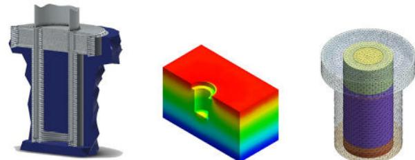
Terracon performs finite element analysis using Midas GTS NX and Plaxis 3D software to model the foundation systems and evaluate the geotechnical and structural capacities of these foundations to support the wind turbine load.
