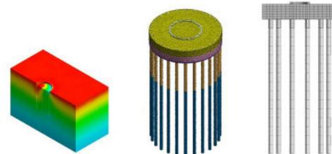
Terracon performs finite element analysis using Midas GTS NX and Plaxis 3D software to model the foundation systems and evaluate the geotechnical and structural capacities of these foundations to support the wind turbine load.
